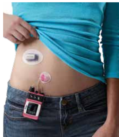
Figure 2. Insulin pump and continuous glucose monitoring (CGM) device in use (Animas Vibe insulin pump and Dexcom CGM device).
