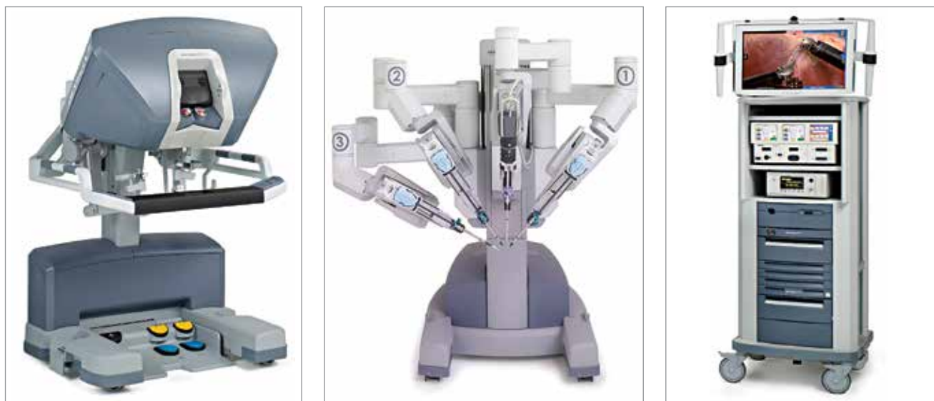
Figure 2. The da Vinci® Surgical System includes three major components: a. (left) surgeon console; b. (middle) patient cart; c. (right) vision cart.
