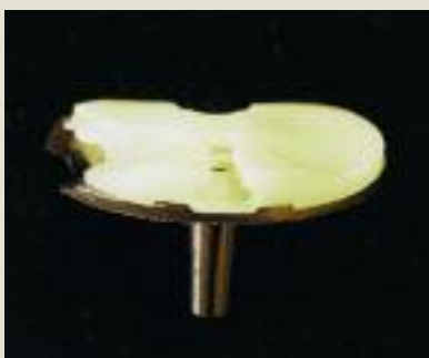
Figure 8 (left). A retrieved specimen with a damaged tibial component from a failed fixed-bearing total knee replacement. The polyethylene insert and the supporting titanium tibial tray are worn on one side. This patient had extensive bone loss as a consequence of particle-induced osteolysis.
