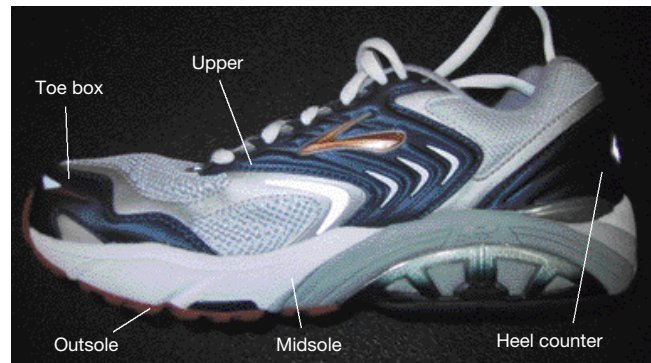
Figure 1. Anatomy of the sports shoe. This shoe has antipronation features of a dual density midsole wedge and a plastic bridge.
