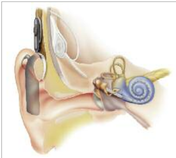
Figure 4. Diagram of the implanted multichannel intra-cochlear electrode and receiver-stimulator unit of a cochlear implant.
